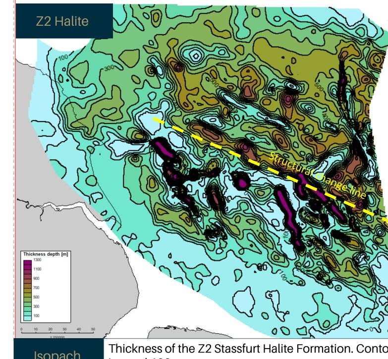
Thickness of the Z2 Stassfurt Halite Formation. Contour Isopach interval 100m
